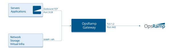
**Option 2.** Telemetry data for compute infrastructure managed by Agents is directly sent to the OpsRamp cloud. Telemetry data for non-compute infrastructure is first sent to the OpsRamp Gateway, which in turn pushes it to the OpsRamp cloud.
